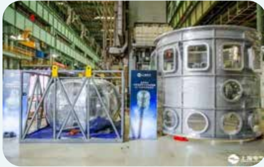
The world's first full high-temperature superconducting Tokamak HH-70 host system
