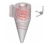
Type A cyclone flue gas flow line diagram
