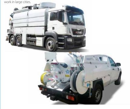
Equipped with multi-function equipment used for emergency rescue, dredging and cleaning operations.
