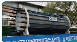
Alkaline Electrolytic Electrolysis
