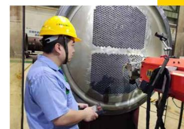
improvements on both the equipment and welding process parameters, they ultimately mastered the critical technology of internal bore welding, providing strong support for the welding manufacturing of the final product.
