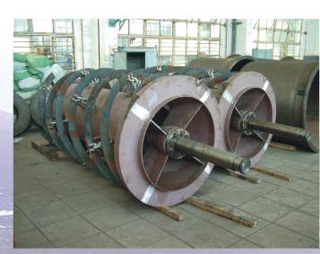
The spiral conveyer consists of spiral propeller and conveyer. One end of spiral propeller connects shell with stay bar, and another end is sustained by bearing outside the shell. The tube rotates spiral propeller when it is running.
