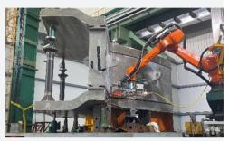
80mm厚度双边激光打底焊 Double Sides Laser Backing Welding with 80mm Thickness
