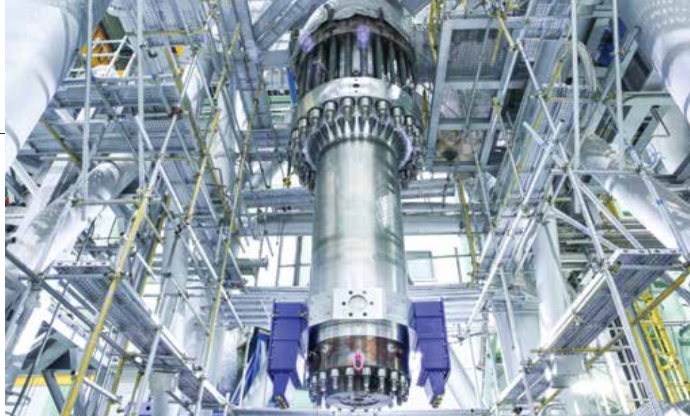
CAP1400湿绕组电机主泵研制成功
